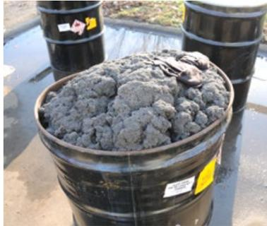
AL Solutions took the raw material from the drums and milled it for several hours in a batch (or lot) while submerging it under water. During milling, a blade reduced the metal particle size and removed the oxide surface layer of the raw material. When milling was completed, operators decanted<sup>3</sup> the water and some fine metal particulates (known as fines) and then sent the water to treatment tanks (Figure 3).
