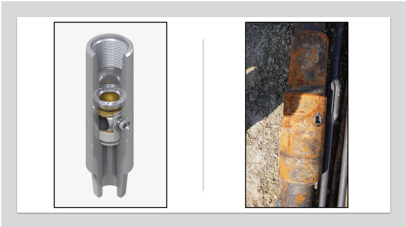
Figure 25. Cutaway view of exemplar FOSV (left) (Credit M&M International [25]) and the FOSV used at the time of the incident (right). (Credit: CSB).
