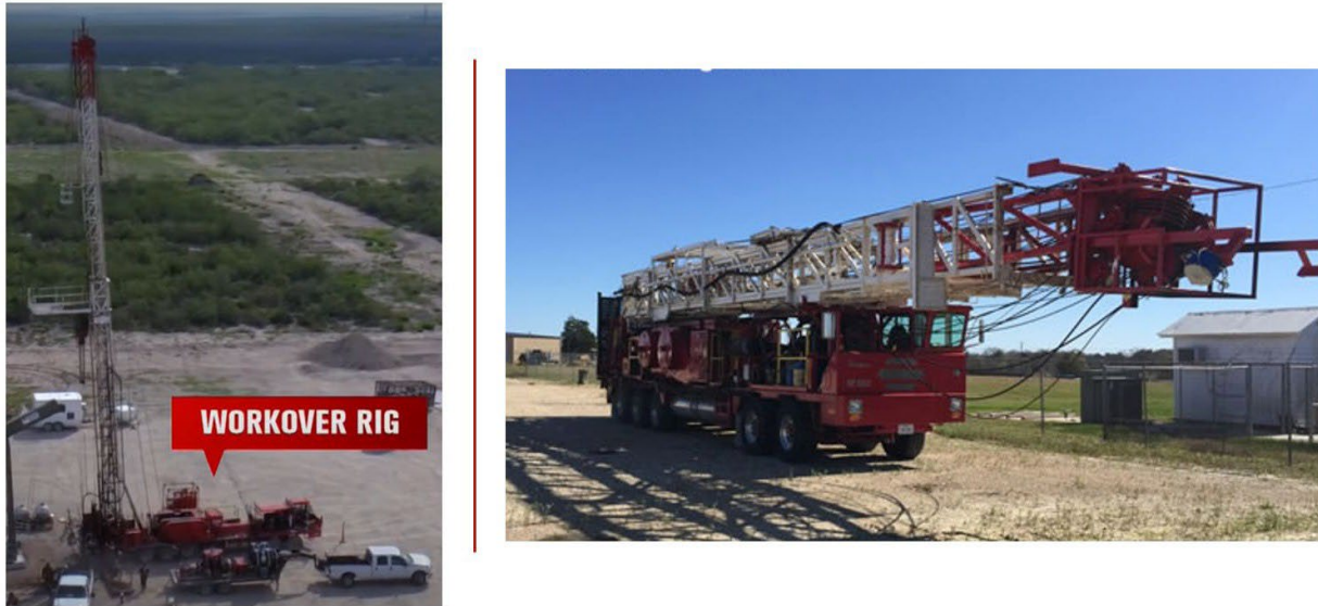
Figure 8. Example workover rig with mast extended (left) and mast stowed (right). (Credit: Dragon Products [left] and World Rigs [right])
