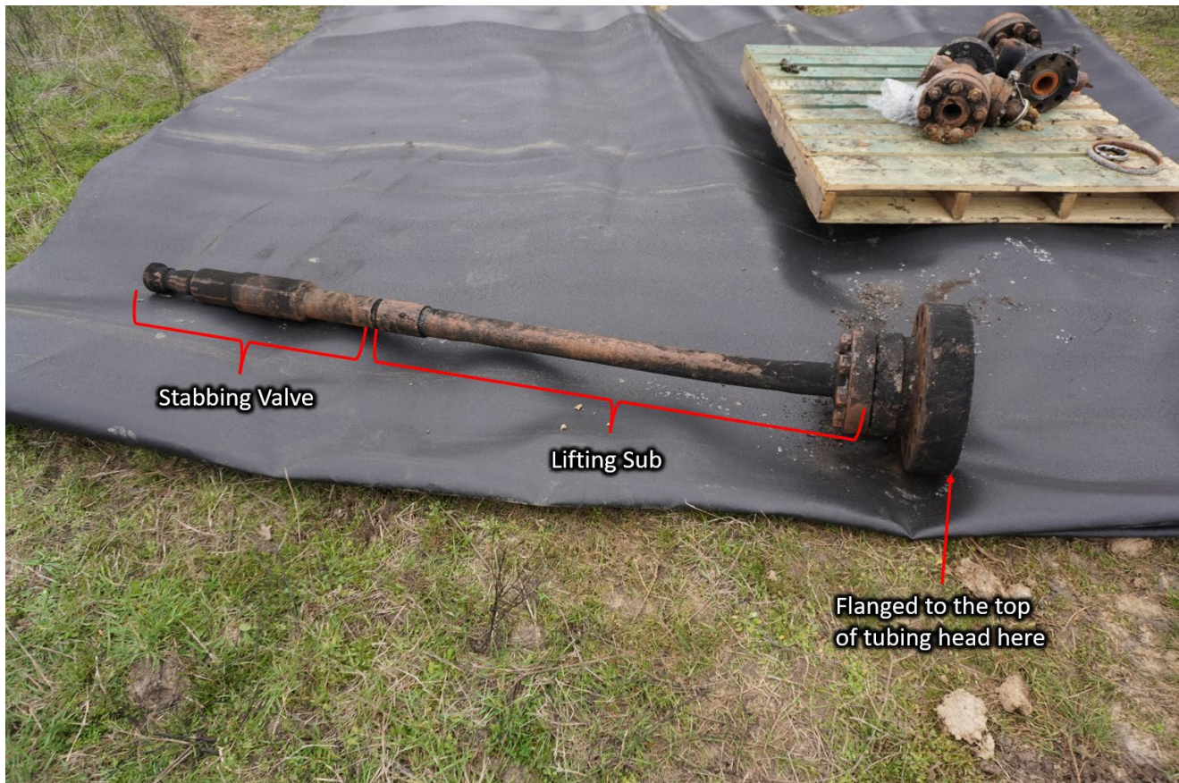
Figure 15. Stabbing valve and lifting sub. (Credit: CSB)
