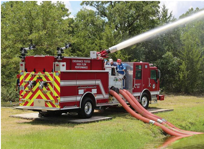
Fire Apparatus Mounted Monitor with Large Capacity Nozzle (S&H Products, Inc.)
