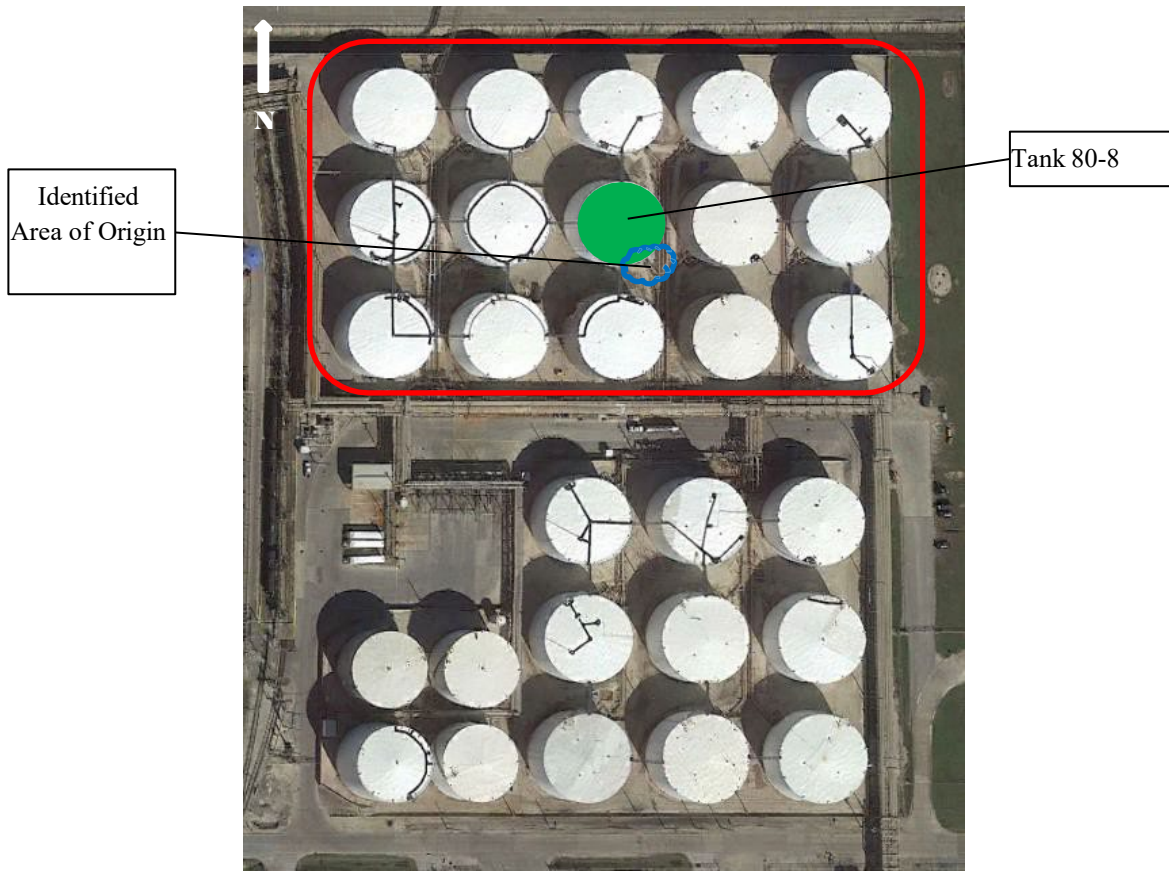
Figure 2: “First and Second 80’s Tank Farm” (Imagery Date: October 28, 2017) [Source: Google Earth Pro] (Tank farm encircled in red. Area of suspected origin identified via blue cloud. Tank 80-8 highlighted in green.)
