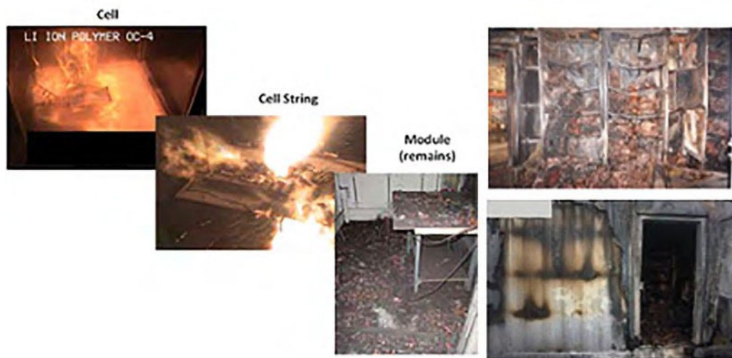
Figure 4.2: Magnified Photos of Fires in Cells, Cell Strings, Modules, and Energy Storage Systems
