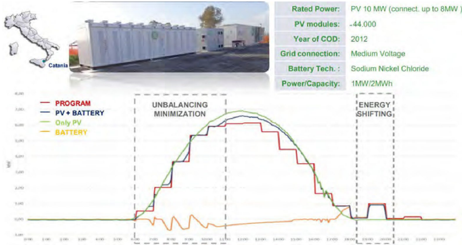
Figure 3.5: Solar Photovoltaic Installation with a Storage System
