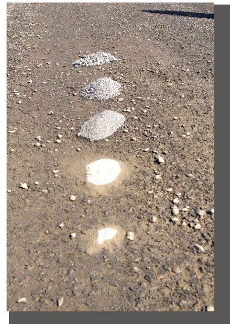
Illustration of the mix of material separated through sieve testing on the road from which the sample was taken.
