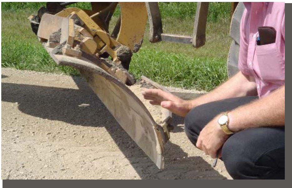
Trainer is demonstrating correct pitch of moldboard for most maintenance operations.
