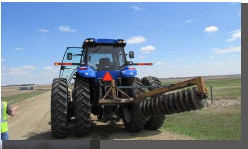
Example of a shouldering disk mounted on a tractor to process sod and gravel before moving it back to the road.
