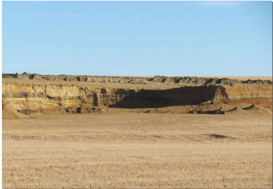
A good example of top soil and vegetation stripped back from the working face of the gravel bank.
