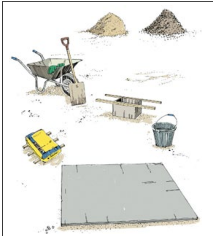
Figure 7. Materials and equipment required for handmixing concrete
