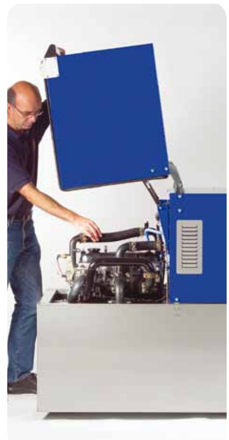
Fig. 3.17: Micro-CHP equipment (internal combustion engine) fuelled by natural gas provides electricity and heat to small and medium premises. The electric efficiency of such devices are not particularly high, but in applications with considerable heating (or cooling) loads this does not matter since the combined electricity plus heat efficiency will be high (Picture: EC Power, Denmark)
