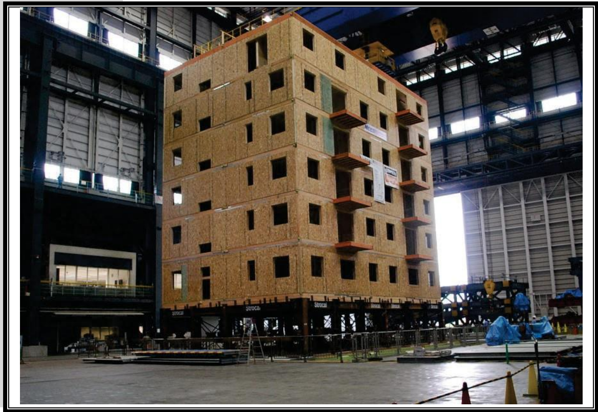
FIGURE 6.2 Six-Story Building on Shake Table, Miki, Japan
